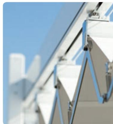
**EN** The transmission system is on load-bearing lateral guides by means of a high-resistance timing belt, rotating on ball bearings. The cast aluminium carter has belt traction regulation. The load-bearing profile (70x130 mm) and the windbreak support bar (40x50 mm) are made of aluminium, while the brackets are in stainless steel and the casting in painted aluminium.
