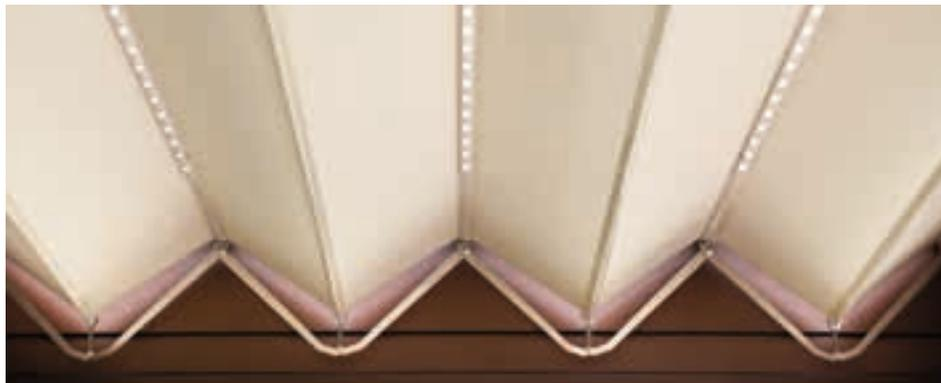
**EN Led Spot integrated in the windbreak bar** (see page 19), with the bar incorporated in the windbreak bar, with groups of 6 leds every 50 cm: **Rectangular led spots** formed of groups of 6 0.5 W leds, for a total of 3 w/spot. Uses around ½ of the light given by the 6 leds. Led Spot can only be installed on Plana fabric systems.
